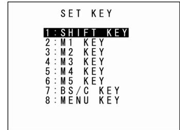
2. Use the cursor keys ([▲] [▼]) or numeric keys ([1] [2] [3] [4] [5] [6] [7] [8]) to highlight the item to be set, and then press the **ENT** key.
