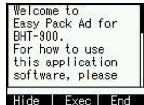
2. Press the **SCAN** key to activate the Easy Pack Ad for BHT-900.
